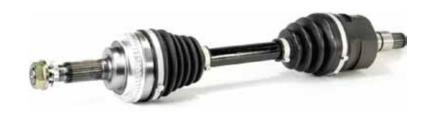
Driveshafts are responsible for transmitting power and torque from the differential to the wheel in automotive applications. Most automotive driveshafts feature Constant Velocity or CV joints, that can articulate and plunge to allow for steering and suspension travel.
